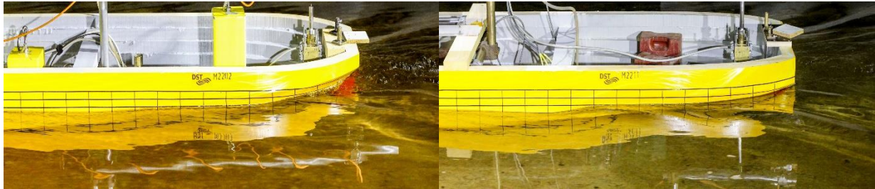
Figure 4: Experimental verification of the optimisation results in DST's large shallow water basin. The smooth ship wake for the new design on the right can be noticed.
