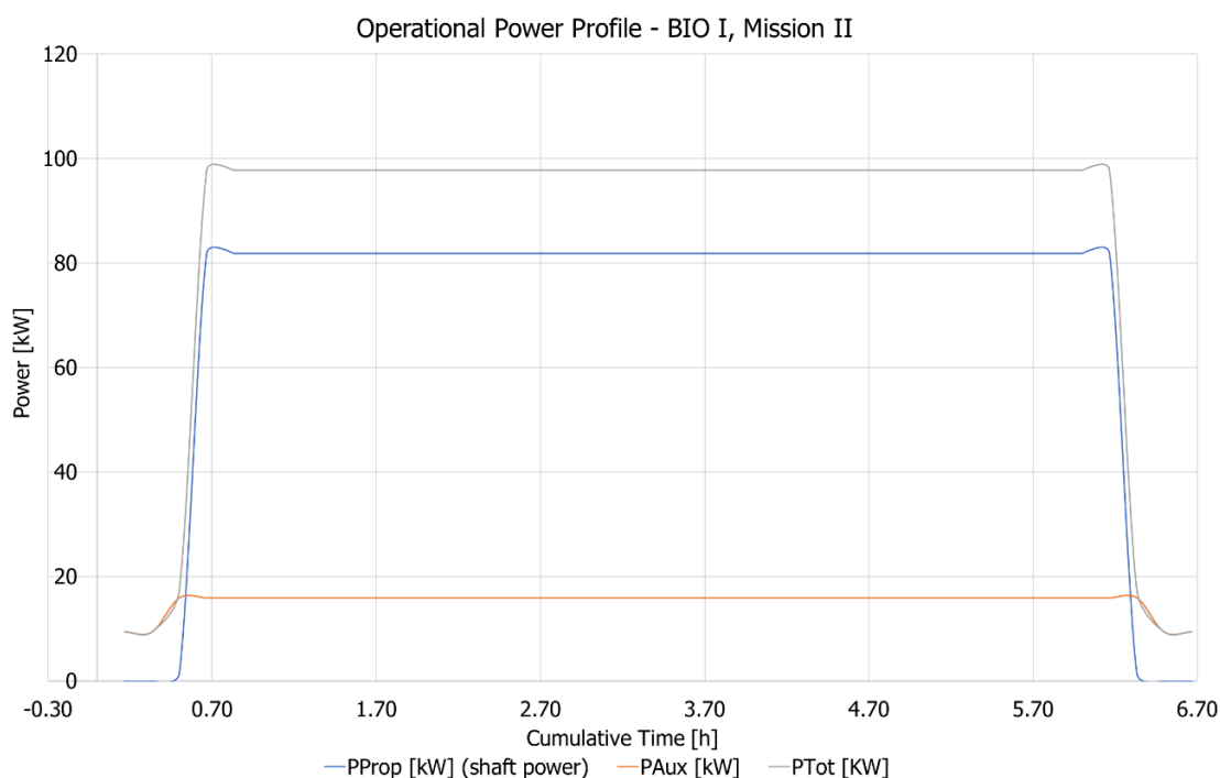
Figure 8-9: Demo 6. Task Power Time Chart, Mission I, BIO I. Sailing from Krems an der Donau to Bad Deutsch-Altenburg.
