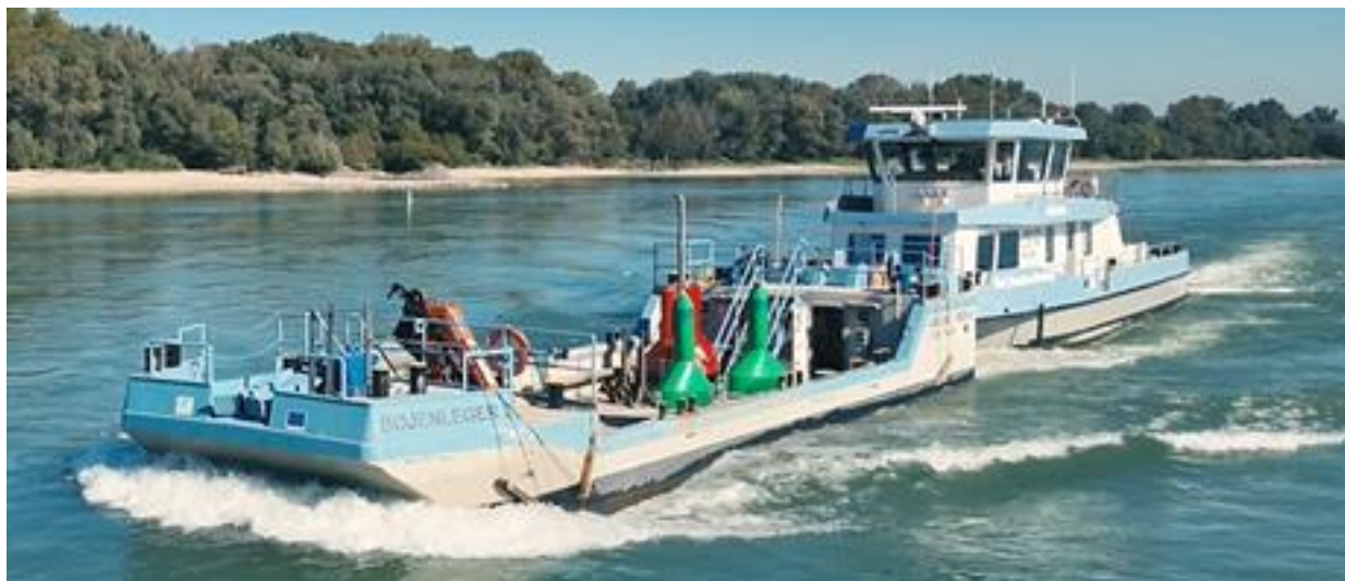
Figure 8-2: The Bad Deutsch-Altenburg pushing a barge carrying waterway marking equipment.
