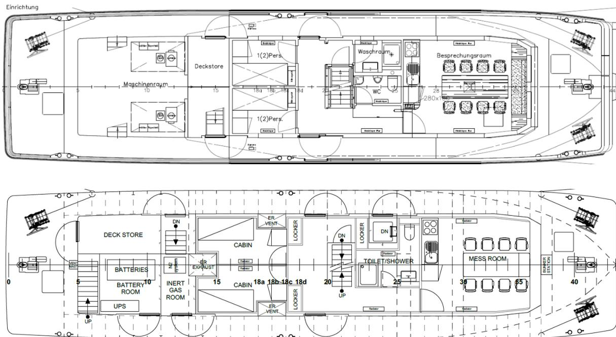
Figure 3-9: Comparison of the spaces on main deck for the Bad Deutsch Altenburg (top) and the new design (bottom).
