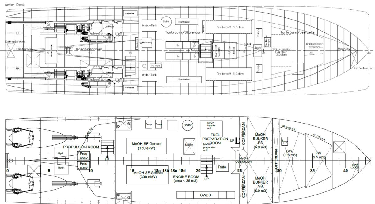
Figure 3-8: Comparison of the spaces below main deck for the Bad Deutsch Altenburg (top) and the new design (bottom).
