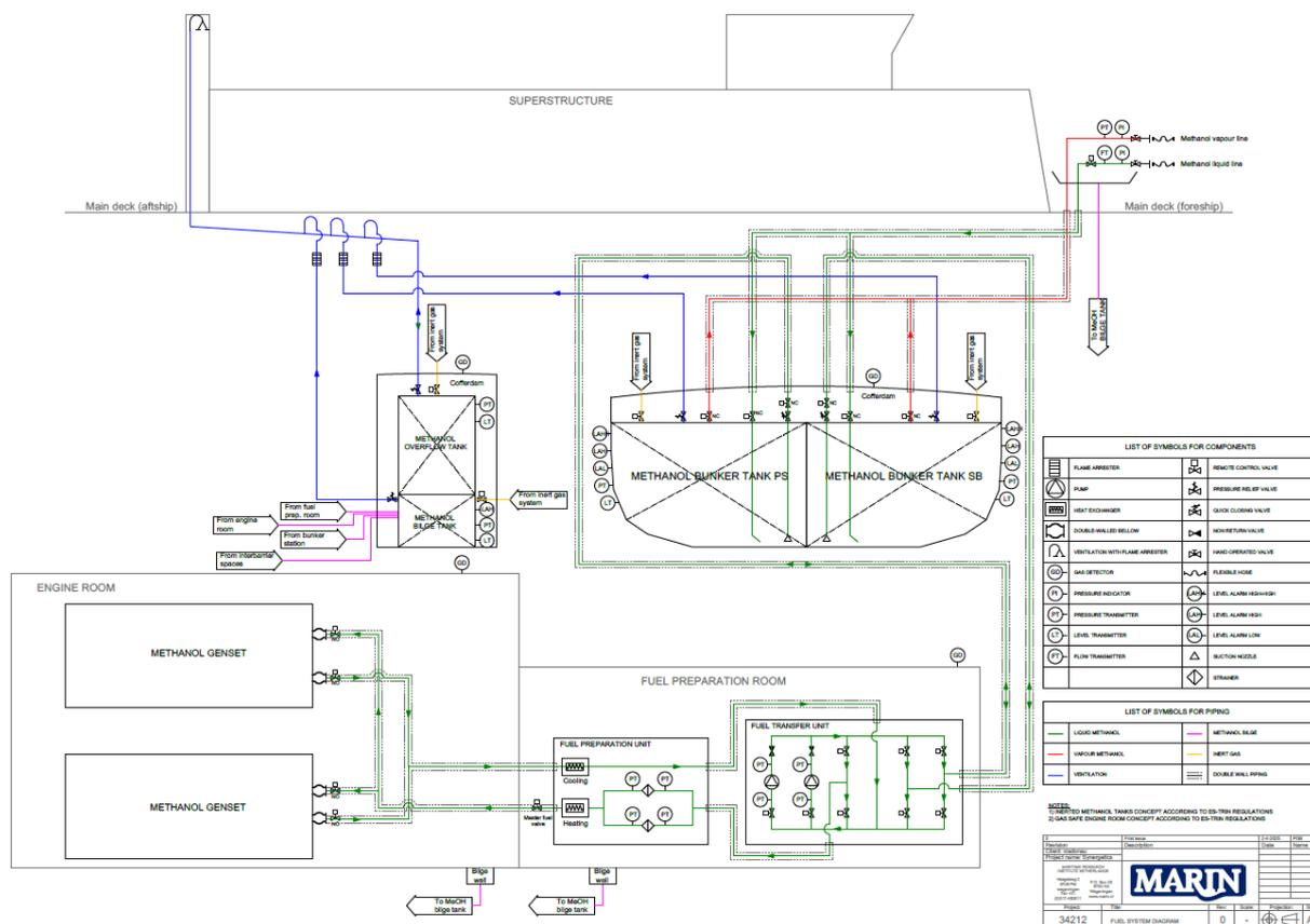
Figure 3-12: Fuel system diagram of the methanol-electric push boat indicating the methanol liquid line (green), methanol vapour line (red), venting/deaeration line (blue) and inert gas line (magenta).
