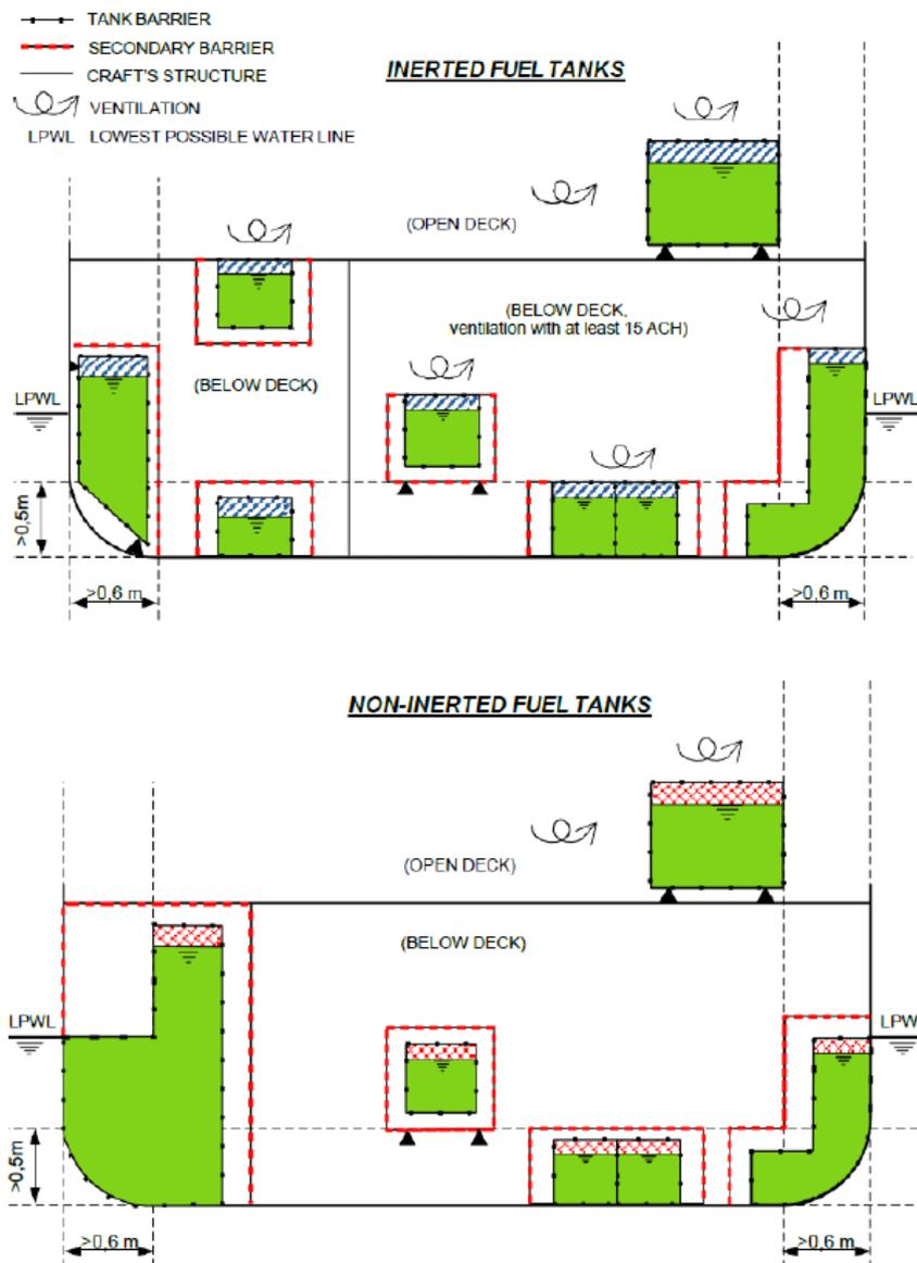
Figure 3-10: Illustration of typical tank arrangements in accordance with ES-TRIN, Annex 8, (2.2.3) and (2.2.4); other configurations are possible
