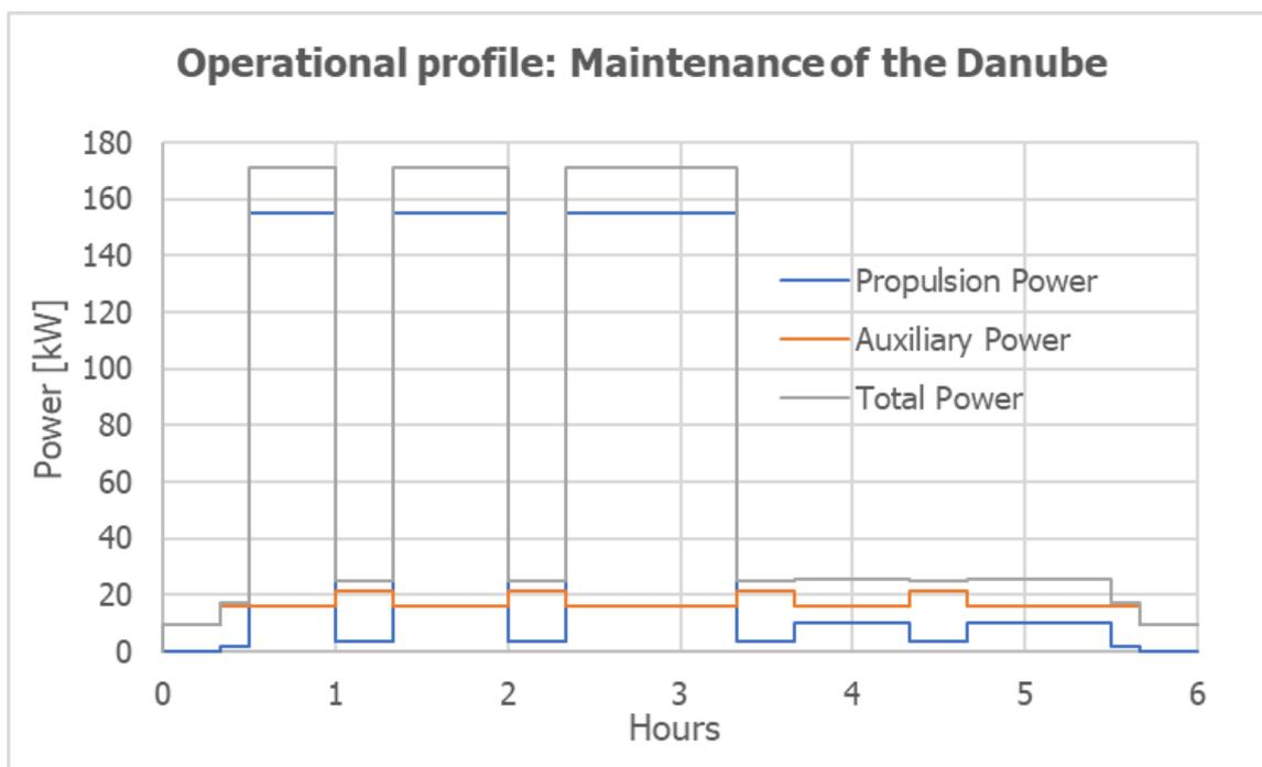
Figure 3-6: Example of a Task Power Time Chart (TPTC) of Demo 6.
