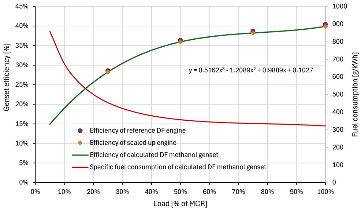
Figure 3-1: Example of the calculated efficiency and fuel consumption for the dual-fuel methanol genset.
