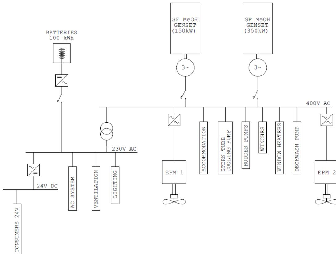
Figure 3-7: Single line diagram of power system architecture SF.2, selected for Demo 6.
