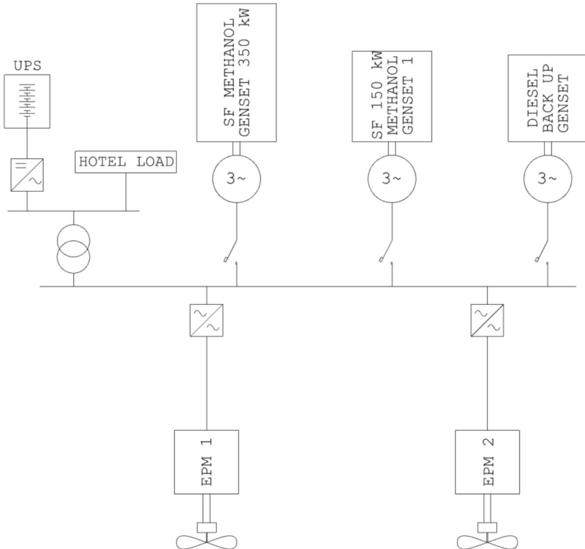
Figure 3-5 Single Fuel Architecture 2
