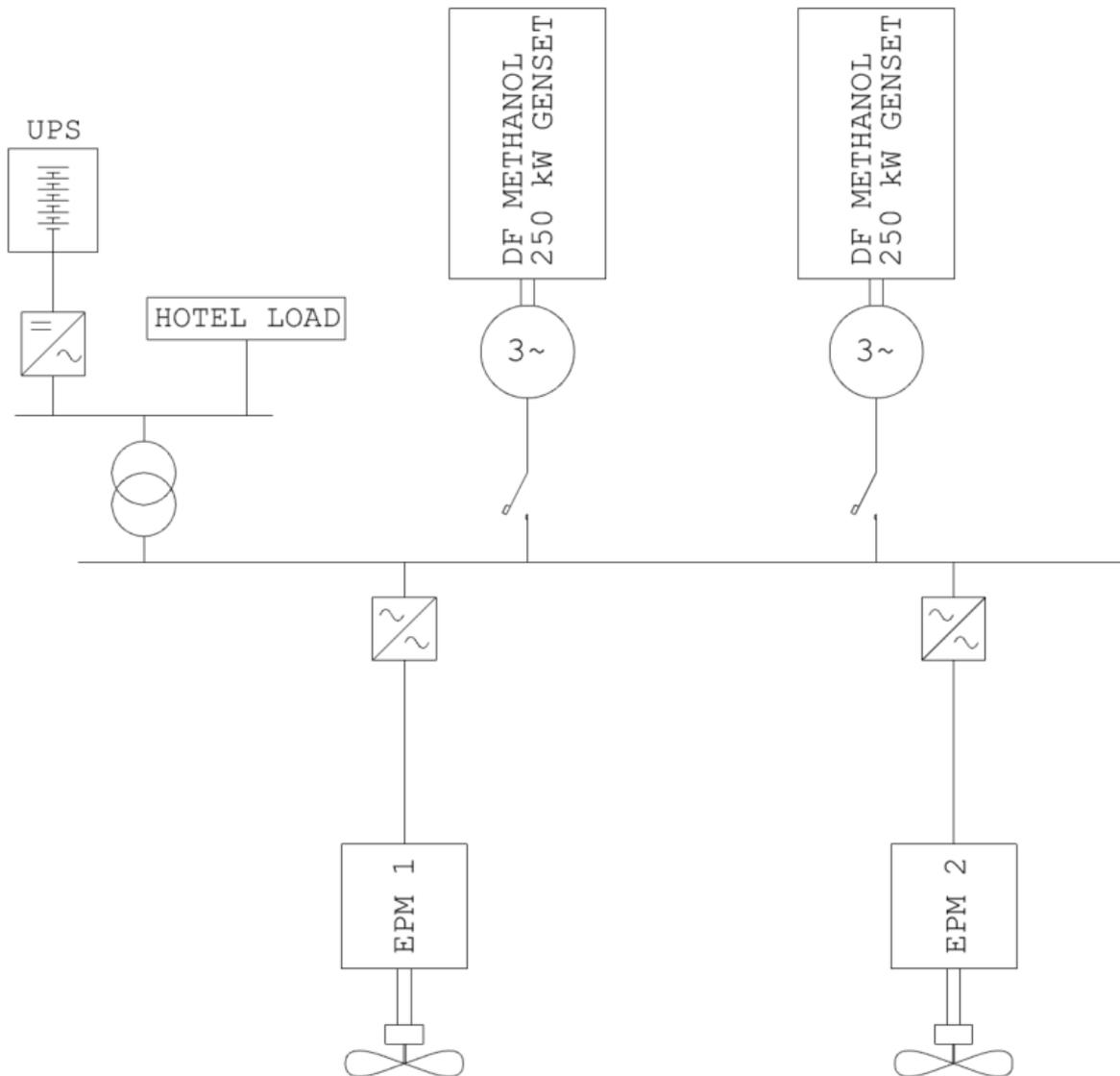
Figure 3-3: Dual Fuel Architecture 2
