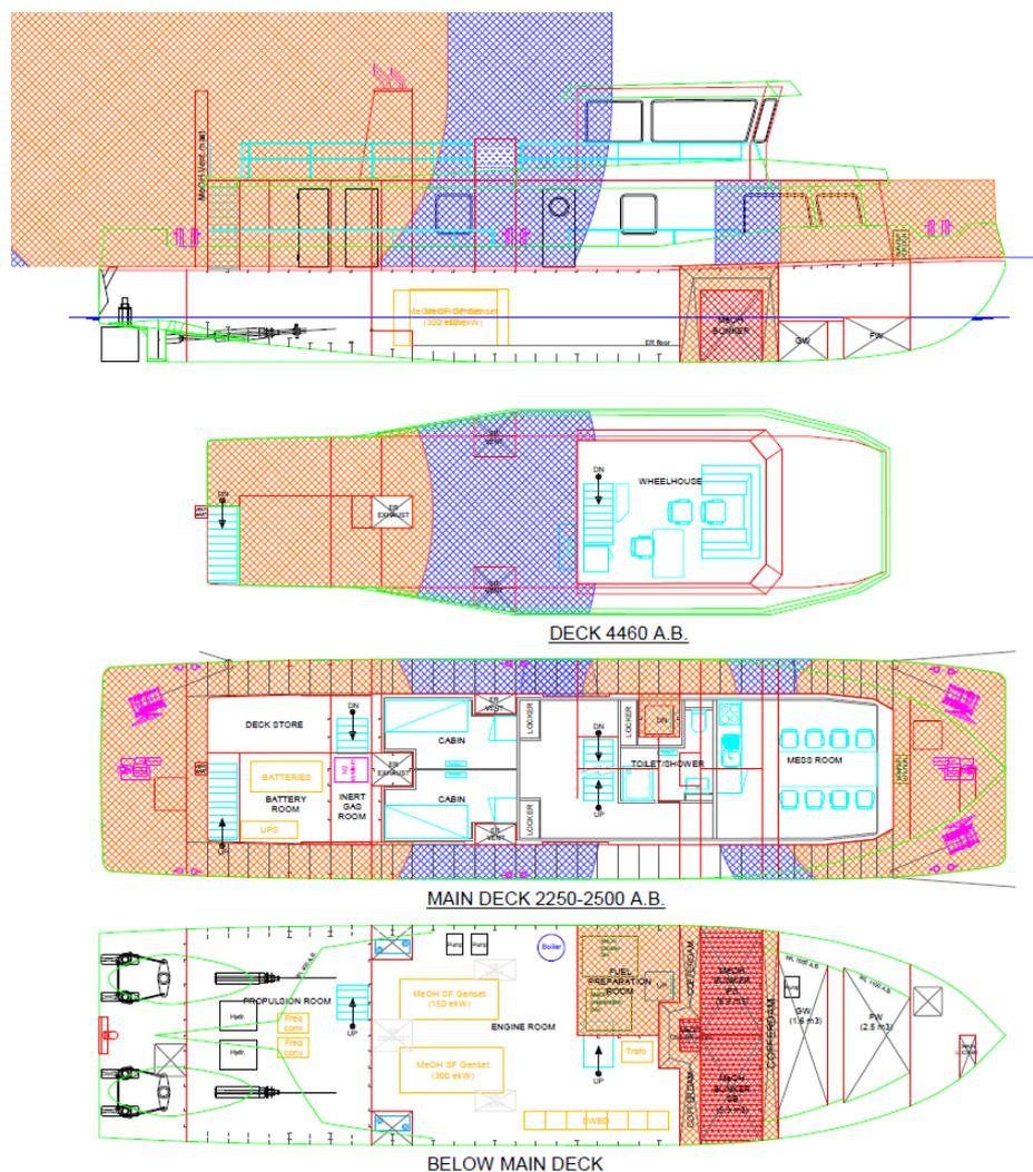
Figure 3-11: Hazardous areas on the methanol-fuelled push boat according to IMO MSC.1/Circ.1621.
