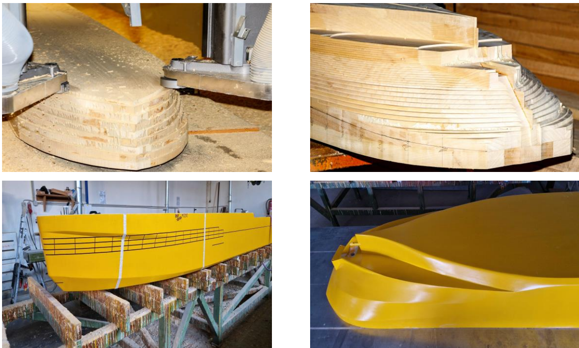
8 | Manufacturing process of the original model geometry (M2202) at DST premises.
