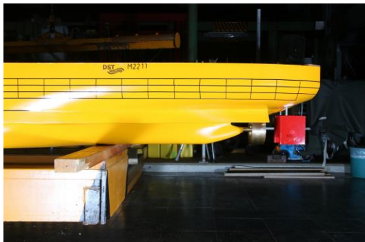
29 | Optimized aft-ship model configuration (M2211) during preparation for testing at DST.
